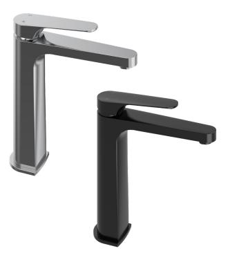
CONSTRUCTION: Solid DR brass PRESSURE: All pressure WORKING PRESSURE (KPA): 35–1000 RECOMMENDED WORKING PRESSURE (KPA): 500 HEIGHT (MM): 266 WIDTH (MM): 231 WATER CONSUMPTION (L/MIN): 6.34 WELS RATING: 4 star rated WATER CONSUMPTION — LOW PRESSURE (L/MIN): 5.84 WELS RATING — LOW PRESSURE: 5 star rated WARRANTY: 10 years on chrome, 2 years on coloured finish, 5 years on cartridge
