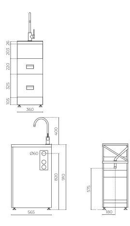
INSTALLATION: Floor-standing WIDTH (MM): 360 DEPTH (MM): 565 HEIGHT (MM): 910 WARRANTY: 5 years on cabinet and all pressure mixer 20 years bowl and ceramic cartridge OVERFLOW / CAPACITY (L/MIN): Yes / Greater than 25 PRESSURE: All pressure WELS RATING: 4 star rated WATER CONSUMPTION (L/MIN): 7.5 TAP HEIGHT(MM): ~ 400
