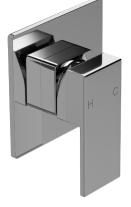
CONSTRUCTION: Solid DR Brass PRESSURE: Mains pressure SUITABLE FOR ALL PRESURE: No WORKING PRESSURE (KPA): 150–1000 RECOMMENDED WORKING PRESSURE (KPA): 500 HEIGHT (MM): 130 WIDTH (MM): 100 WARRANTY: 10 years on chrome, 2 years on coloured finish & 5 years on cartridge DIVERTER: No
