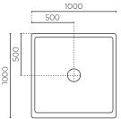
CONSTRUCTION: Acrylic WIDTH (MM): 1000 DEPTH (MM): 1000 HEIGHT (MM): 1940 DOOR/S: 1 SHAPE: Square TRAY UPSTAND (MM): 35 WASTE LOCATION: Centre MOULDED: No WARRANTY: 10 years on Acrylic walls, tray and doors, 2 years on shower seals
