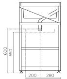
INSTALLATION: Floor-standing WIDTH (MM): 560 DEPTH (MM): 565 HEIGHT (MM): 910 WARRANTY: 5 years on cabinet and all pressure mixer 20 years bowl and ceramic cartridge OVERFLOW / CAPACITY (L/MIN): Yes / Greater than 25 PRESSURE: All pressure WELS RATING: 3 star rated WATER CONSUMPTION (L/MIN): 9 TAP HEIGHT(MM): ~165
