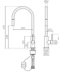
**CONSTRUCTION:** Stainless steel **PRESSURE:** Mains pressure WORKING PRESSURE (KPA): 150-1000 **RECOMMENDED WORKING PRESSURE (KPA):** 500 HEIGHT (MM): 425 WATER CONSUMPTION (L/MIN): 5.58 WELS RATING: 5 star rated WARRANTY: Lifetime on stainless steel, 5 years on coloured finish, 5 years on cartridge **LEAD FREE:** Yes
