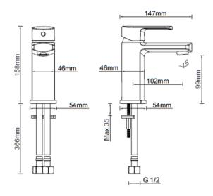
CLASSIFICATION: Suitable for all pressures INLET CONNECTIONS: 1/2 " BSP WORKING PRESSURE: 35 - 500kPa OPERATING TEMPERATURE: 5 °C - 80 °C
