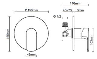
CLASSIFICATION: Suitable for all pressures INLET CONNECTIONS: 1/2 " BSP WORKING PRESSURE: 55 - 500kPa OPERATING TEMPERATURE: 5 °C - 80 °C
